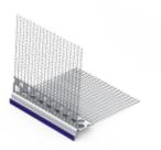
The profile with under drip is used for clean finish of the window edge in the thermal insulation system. This variant has visible eaves strip and ensures dripping of water in the vertical direction which prevents the wicking of water into the structure. It is made of PVC material and glued glass fiber grid.
