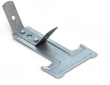
The bracket is used for a quick mounting of drywall steel profiles CD 60 into a horizontal construction of the building. It is produced by compression molding of rolled galvanized metal sheet with thickness of 0.80 mm and single spring clip which is pressed into the hanger with two rivets. The installation is done by sliding into the profile and subsequent hanging on the suspension wire which allows a quick and easy leveling of the construction.
