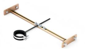
Sanitary support for drain pipe is construction element which is produced by compression molding and sheet metal sections of "C" shape. The metal profiles are attached to side plate-by welding and thus form two sliding spacers. To maintain the required resistance in humid environments, both structures are after welding protected with yellow (standard) or blue (on request) galvanized zinc. Fasteners provide attachment to the structure and fixing spacers.
