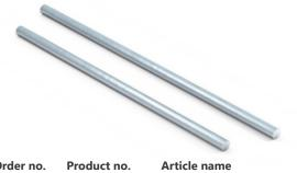
The element is made of galvanized steel wire with diameter of 4.00 mm. It is used for extended suspension of the steel drywall or main profile structures into solid construction of the building. Quick hanger or butterfly spring can be mounted on the straight end of the wire.
