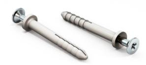
The nail plug is used for anchoring the wooden laths, beams, steel profiles into an existing support structures of solid building materials. The product consists of the nylon plug and the steel nail. It allows the quick and easy installation by hammering
