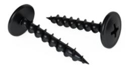
The screw is used for mounting of metal drywall accesories into the wooden structure. It is produced in several length variations with a coarse thread, flat head and phosphate surface.
