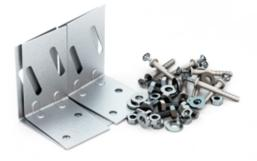
The angle is used for anchoring the drywall steel profiles UA into a construction of the building in vertical system. It is produced by compression molding of rolled, galvanized metal sheet with thickness of 1.50 mm. The element is attached into a construction by nail plugs and into the UA profiles by metric screws. The angle can be also used for fastening a steel door frame.
