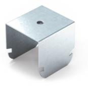
The cross connector is used for mounting the double cross grid created from drywall steel profiles BA 50 or BS 50. It is produced by compression molding of the rolled galvanized steel sheet with a thickness of 1.00 mm in variant with a hole of 6 mm or a thread M6. To simplify the work it is supplied already bendet state and it is secured by snapping into the profile.
