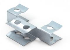
The clip is used for level connection of two gypsum boards with thickness of 9.5 mm. It is produced by compression molding of the rolled galvanized steel sheet with a thickness of 0.60 mm.
