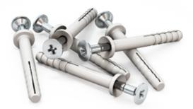
The nail plug is used for anchoring the wooden laths, beams, steel profiles into an existing support structures of solid building materials. The product consists of the nylon plug and the steel nail. It allows the quick and easy installation by hammering into a pre-drilled hole
