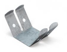
The butterfly clip is used for connecting two suspension wires in a drywall construction. It is produced by compression molding from spring metal sheet with thickness of 0.60 mm which is covered by anticorrosive Delta Protekt surface. The element allows very simple and highly variable reduction of the ceiling.
