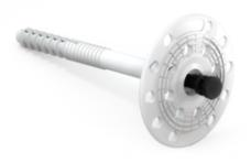
The dowel is used as an anchoring element for fixing insulation boards in thermal insulation system. It is made from quality materials in several lengths. Installation into the structure is performed by inserting into prepared hole and hammering the plastic mandrel.
